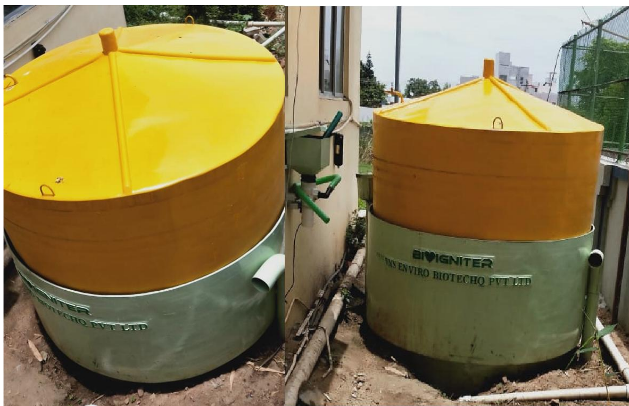
Figure 3: Biogas Plant of capacity 5m3 per day
