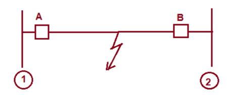
In case of fault, breaker A and B should open. Let us assume that, the fault is being sensed by relay at station 1. This relay should issue trip command to breaker A and send trip signal to the remote end. This trip signal to remote end is called Direct Trip(DT) signal.
