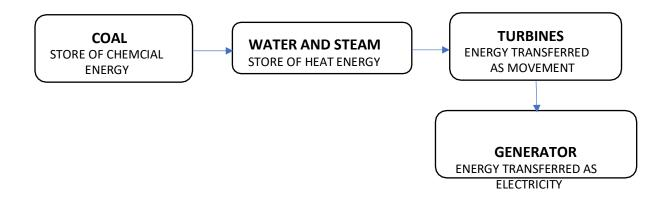
Its operation involves the production of super-heated steam in the boiler which rotates the turbine where the mechanical energy gets converted into electrical energy. The basic raw materials are coal and water.
