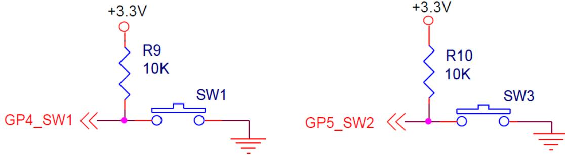
GPIO 4 & GPIO 5, can be used as an Input Pin and connected to a simple momentary push button switch pulled up through a 10K Resistor, as shown above. So, normally the Pico reads HIGH on the button pin but when the button is pushed, Pico reads LOW on the button pin.
